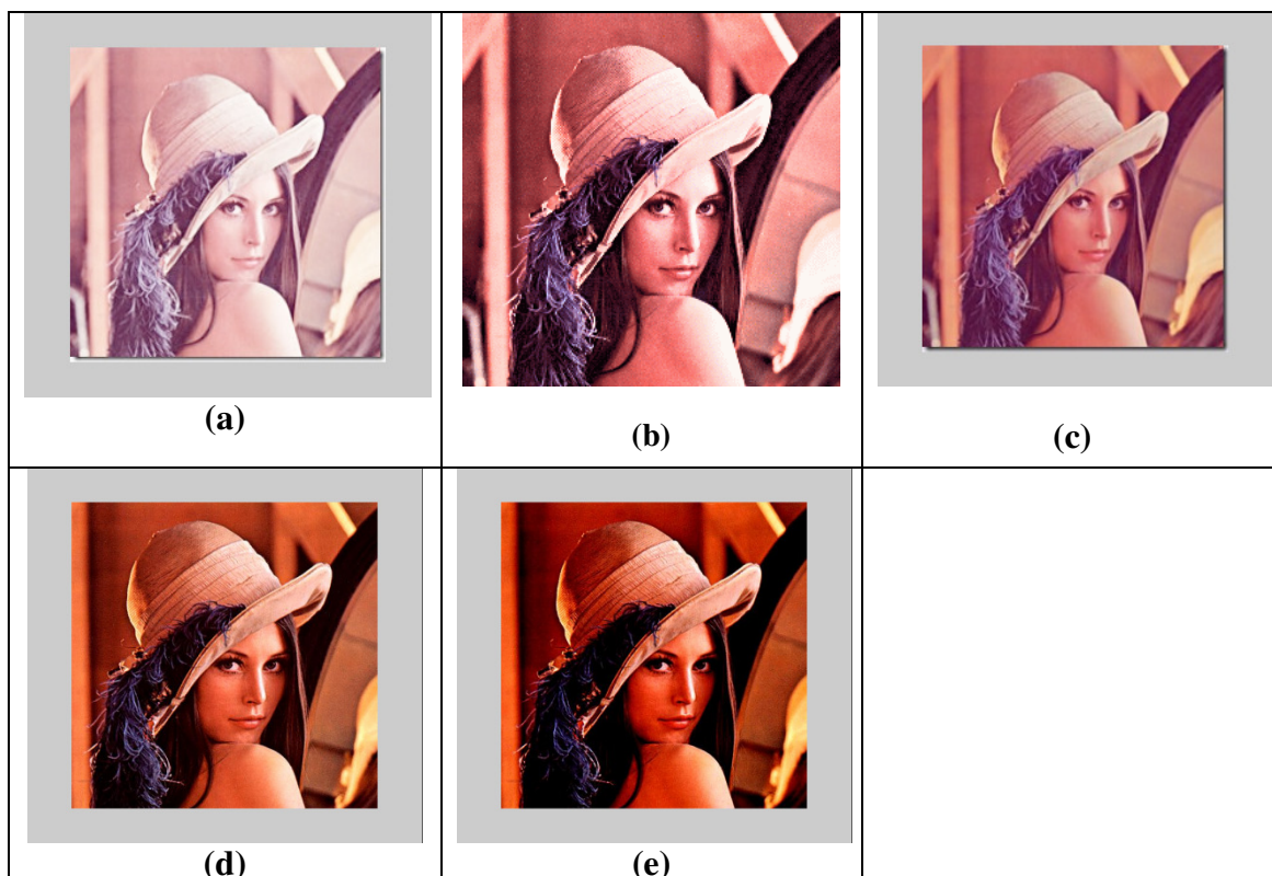
Figure (5.9) : Saturation enhancement of Luna image (a) Original image. (b) Pei's method [20] applied to (a). (c), (d) and (e) Application of the proposed method, SSGA, to (a) The saturation transfer function f(r) as Fig. (4.7) with empirical parameters as shown in table (5.3).
