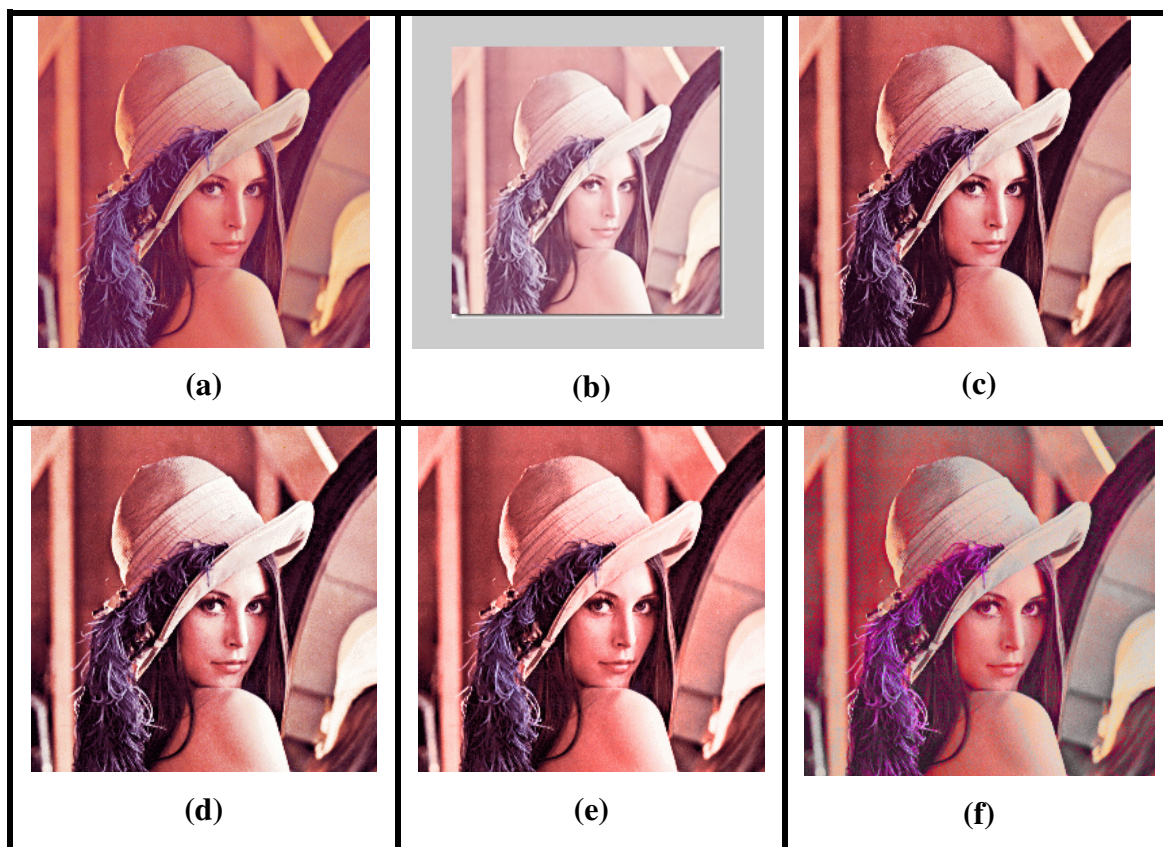
Figure (5.3) : Results on Luna image. (a) Original Image (b) proposed method (SSGA) (c) S-type enhancement with n = 2 and m = 1.5 , (d) histogram equalization (e) Yang et al.'s method in LHS system, and (f) Weeks et al.'s method.
